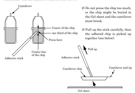
Note: Some of both-side adhesive tapes have not enough adhesive to pick up the chip from the Gel sheet. Then use the tweezers for this procedure.
