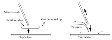
Note) To avoid contact with the cantilever. the tweezers should not access to the chip from cantilever side. Put the tweezers on the chip like following illustration.
