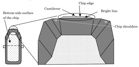
Schematic view of cantilever chip
