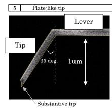
Left image is an SEM image of the cantilever apex viewing from the side. The plate-like tip is located at the end of the cantilever.
