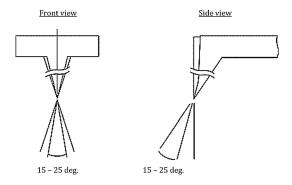
Sharpening effect around tip apex
